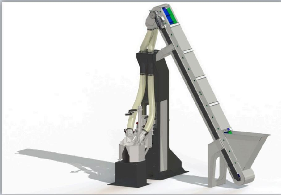
At the heart of our innovation is the Potting Module and Soil Conveyor, a key component in our system's development. This module efficiently handles the transport of potting soil while securely anchoring trees in place, making it a central part of the potting process.
