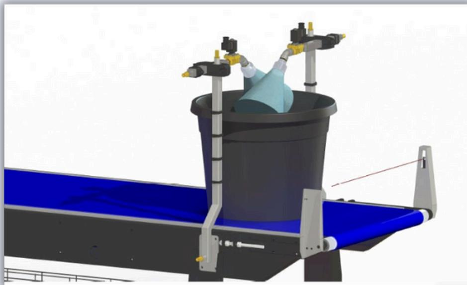
The Watering System option is integrated into the process to ensure that plants receive the necessary watering while waiting on the Tree Output Conveyor. This immediate watering benefits the plants, as they would otherwise need to wait until reaching their final destination in the nursery or be watered.
